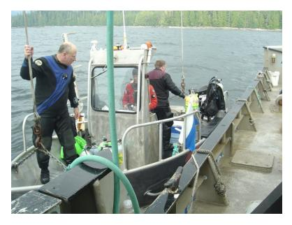
Research divers operate out of two skiffs that have been fitted with racks, tank holders, depth finders, and a GPS to aid in navigation and diving.
